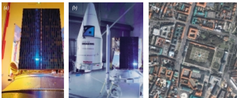
Figure 1: (a) An IKONOS satellite being checked out in a clean room at Lockheed Martin. (Source: Lockheed Martin) (b) An IKONOS satellite sitting alongside its protective nose cone. It was the failure of this protective cover to separate from the Athena launcher that caused the loss of the IKONOS-1 satellite in April 1999. (Source: Lockheed Martin), (c) A multi-spectral IKONOS image of part of the city centre of Munich, Germany. (Source: Space Imaging)
