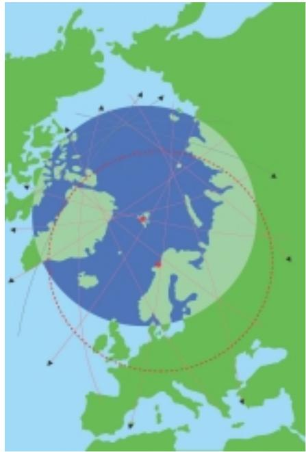
Showing the orbital tracks of a polar orbiting satellite relative to the coverages of the Tromsø & Svalbard ground stations. (Source: Norwegian Space Centre)
