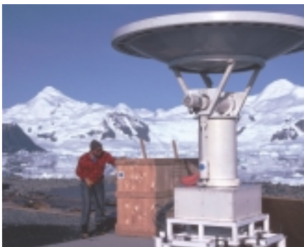
The ARIES (Antarctic Reception Imagery for Environmental Studies) antenna located at the Rothera Base of the British Antarctic Survey (BAS) for the acquisition of HRPT weather imagery from NOAA satellites, prior to the erection of its radome. (Source: BAS; Photographer: P. Bucktrout)
