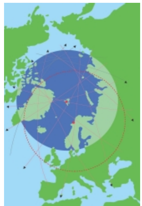
Showing the orbital tracks of a polar orbiting satellite relative to the coverages of the Tromsø & Svalbard ground stations. (Source: Norwegian Space Centre)
