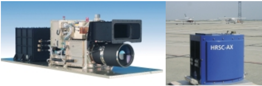
Fig. 6 - (a) DLR's HRSC 3-line pushbroom scanner as deployed on the Mars Express mission. (b) The HRSC-AX airborne version of the HRSC 3-line pushbroom scanner. (Source: DLR)
