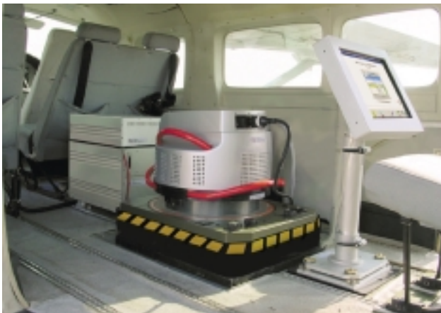
Fig. 7 - The Leica Geosystems ADS40 airborne 3-line pushbroom scanner as deployed operationally in an aircraft. (Source: Leica Geosystems)
