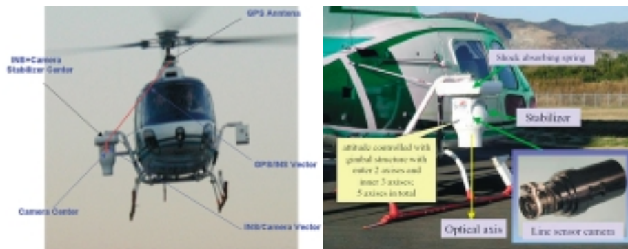
Fig. 8 - (a) The Starimager system mounted on a helicopter, showing the positions of the various system components on the aircraft. (b) A close-up view of the Starimager 3-line pushbroom scanner on its stabilized gimbal mount attached to the side of its helicopter platform. (Source: Inst. of Geodesy & Photogrammetry, ETH, Zürich)
