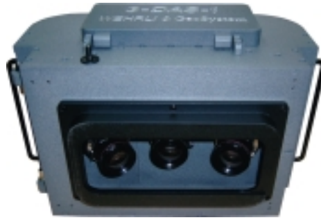
Fig. 9 - (a) An overall view of the Wehrli 3-DAS-1 3-line pushbroom scanner sitting on its ASP-1 stabilized mount. (b) A close-up view of the underside of the Wehrli 3-DAS-1 pushbroom line scanner with its three lenses as seen from below. (Source: Wehrli Associates)
