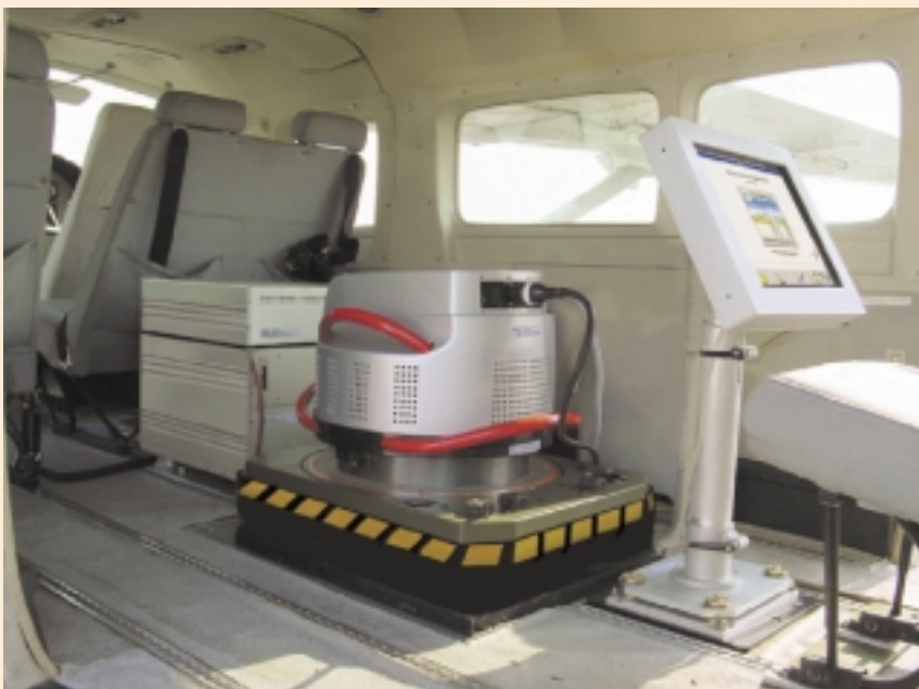
Figure 8: (c) The ADS40 (Source: LH Systems) airborne pushbroom scanner system.
