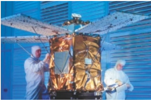
2. (a) The OrbView-4 satellite under test at Orbital's facility in Germantown, Virginia. (b) An artist's impression of the OrbView-4 satellite as it will appear in flight. (Source: ORBIMAGE)
