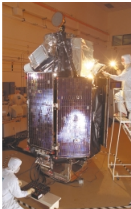
1. (a) The QuickBird-1 satellite under test in a clean room at Ball Aerospace in Boulder, Colorado. (b) An artist's impression of the QuickBird satellite operating in space. (Source: EarthWatch)
