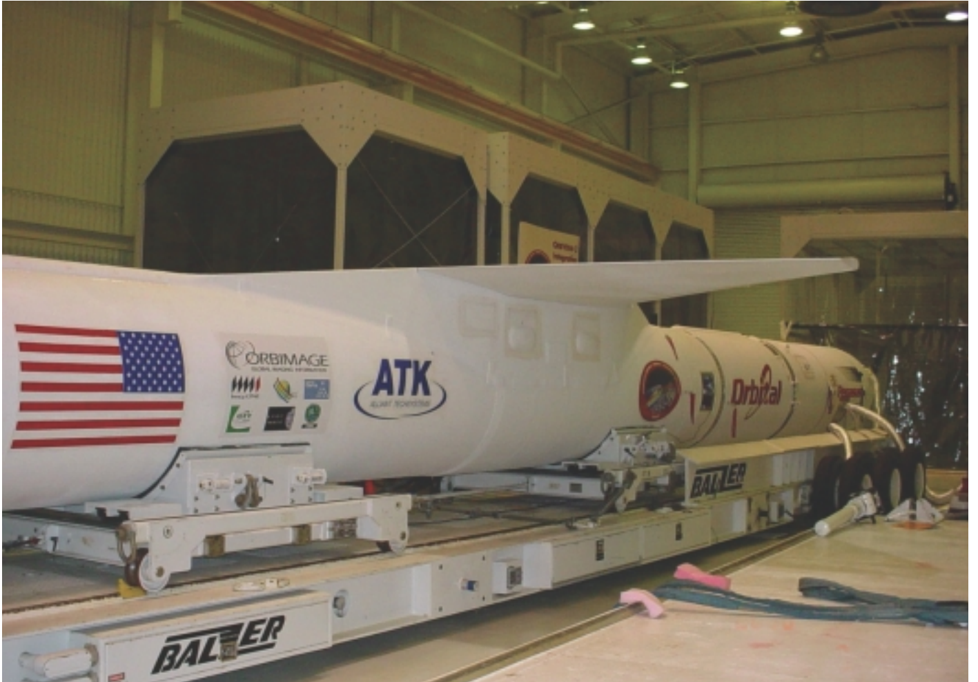
The air-launched Pegasus rocket with its tiny delta wing. The front part of the rocket houses the OrbView-3 satellite, which is covered by a protective fairing.
