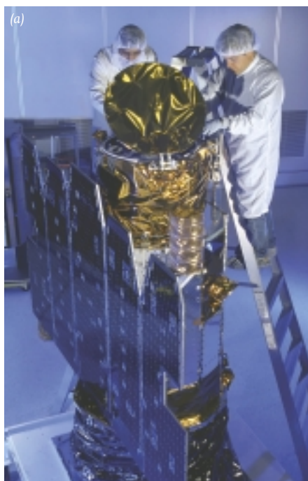
(a) The OrbView-3 satellite being checked out in a clean room at the Orbital Sciences Corporation's facility in Virginia.
