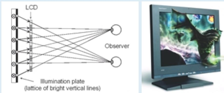
Figure 7: (a) The basis of the DTI 3D auto-stereoscopic display. (b) DTI's 15 inch and (c) 18 inch display monitors (Source: Dimension Technologies Inc.)
