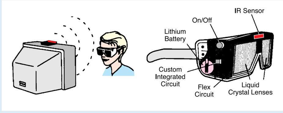
Figure 5: Alternating images on the monitor screen with alternating shutters for 3D stereo-viewing (Mike Shand)
