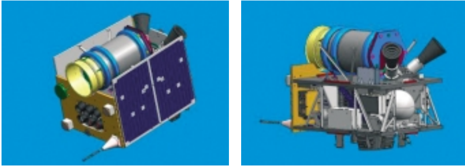
Figure 8 - (a) A CAD drawing providing an external view of the China DMC+4 micro-satellite, including its optical telescope, solar panels and antenna. (Source: SSTL), (b) A CAD drawing with the outer panels removed to show the internal arrangement of the power supply, electronics, etc. within the China DMC+4 micro-satellite. (Source: SSTL)
