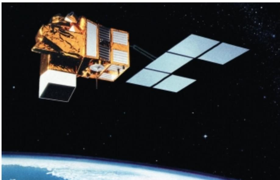
Figure 2 - An artist's impression of one of the forthcoming Helios-2 military high-resolution reconnaissance satellites. The similarities of the basic platform with that of the SPOT-5 satellite [in Fig. 1(b)] can be seen. (Source: Astrium)
