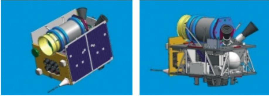
Figure 8 - (a) A CAD drawing providing an external view of the China DMC+4 micro-satellite, including its optical telescope, solar panels and antenna. (Source: SSTL), (b) A CAD drawing with the outer panels removed to show the internal arrangement of the power supply, electronics, etc. within the China DMC+4 micro-satellite. (Source: SSTL)
