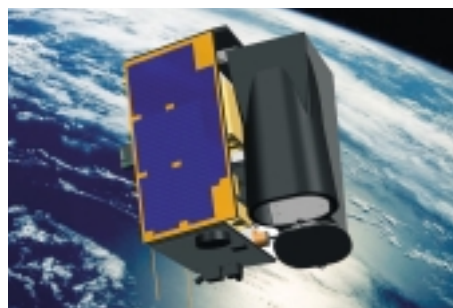
Figure 7 - (a) An artist's impression of TopSat in orbit, showing how the telescope of the high-resolution imager is mounted externally on top of the main body of the micro-satellite. (Source: SSTL)
