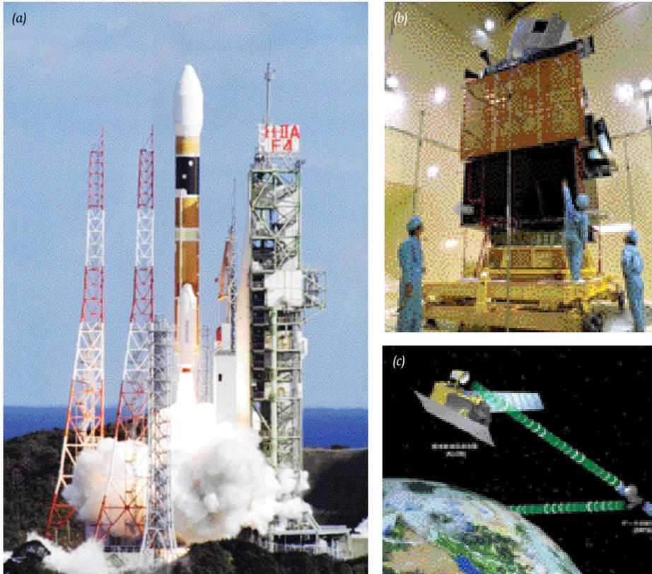
Figure 7. (a) An H-IIA launcher lifting off from the main Japanese launch site at Tanegashima Space Center. (b) The ALOS satellite undergoing tests. (c) An artist's impression of the ALOS satellite in its polar orbit transmitting data via a DRTS communications relay satellite (operating in a geostationary orbit) onwards to a ground receiving station in Japan. (Source: JAXA)
