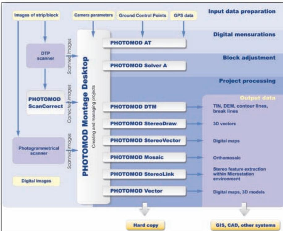
Fig. 2 - A diagram showing the modules and work flow of the PHOTOMOD system, including the input and output data.
