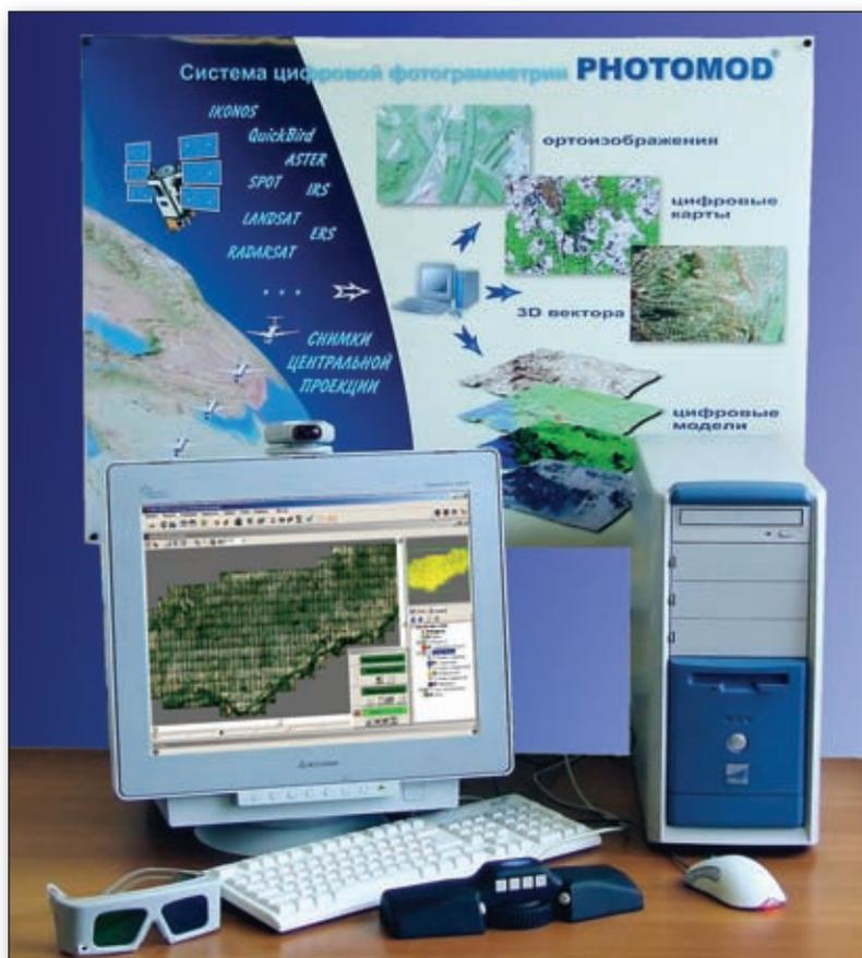
**Fig. 1** - A PHOTOMOD system showing the main hardware components - with the wireless glasses, keyboard, 3D mouse and standard mouse in the foreground; and the display monitor and computer in the middle - with a display board acting as the background.
