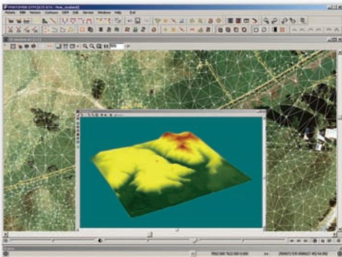
Fig. 3 - A screen shot of the DTM module in use, showing a TIN (Triangular Irregular Network) connecting the measured elevation points superimposed on the image of the corresponding orthophoto. The inset window shows a perspective block diagram of the terrain constructed from the measured DEM.
