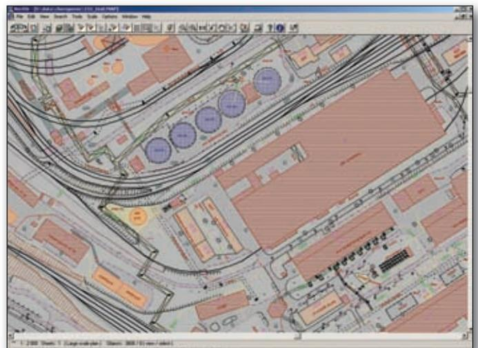
Fig. 4 - The VectOr module is used to edit and annotate the vector features that have been measured using PHOTOMOD and create the final map.
