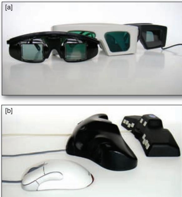
**Fig. 6 (a)** - Examples of the "active" 3D stereo-viewing glasses that can be used with PHOTOMOD showing (from front to back) the wireless E-D glasses from eDimensional; the wireless NuVision 60GX glasses from MacNaughton; and the wired 3D glasses from the Russian supplier, IBIK.
