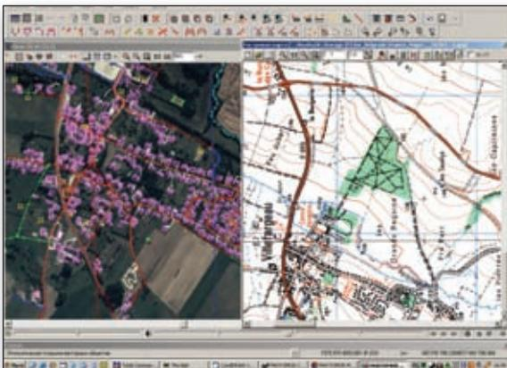
**Fig. 9** - A representative screen shot of the work being undertaken at Racurs for the BD Topo project of IGN France with an annotated othophoto image being displayed alongside an existing map.
