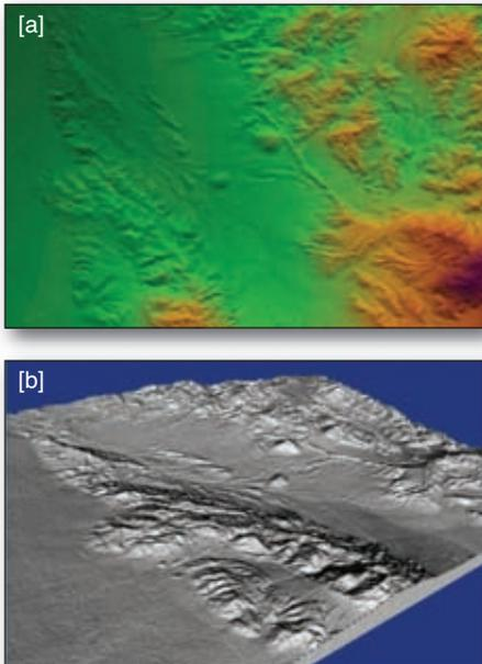
**Fig. 5 (a)** - A digital elevation model (DEM) generated using the stand-alone PHOTOMOD Radar software package.
