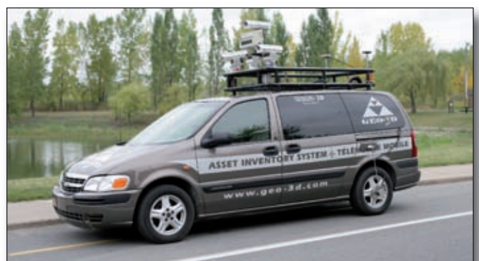
Fig. 4 – The Trimble Road Asset Inventory System is based on the Geo-3D Trident mobile mapping system.
