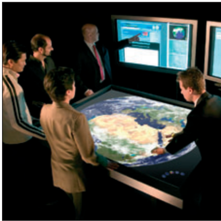
The TouchTable TT84 is seen here being operated by a group standing around its horizontal display surface during a consultation in a boardroom. The two auxiliary vertical plasma display screens can be seen mounted on stands at the back of the main horizontal display surface. (Source: Applied Minds Inc.)
