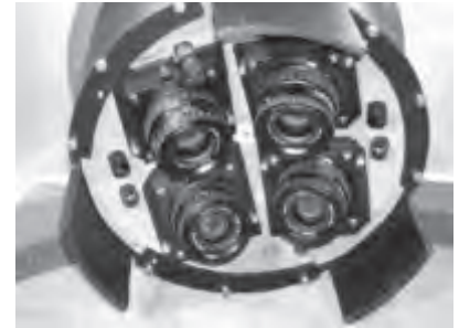
Figure 8. The Rolleimetric AIC x4 system, showing the four oblique pointing AIC medium-format digital cameras.
