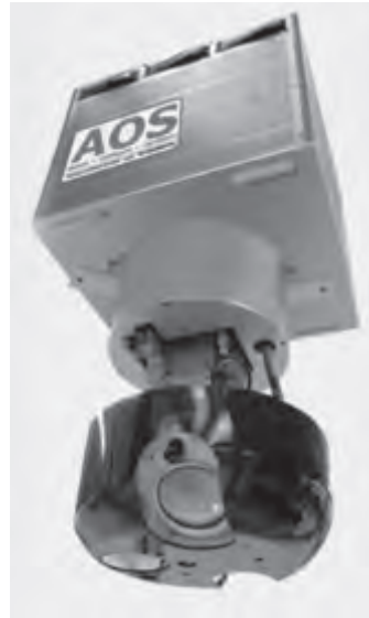
Figure 14. (a) The Rolleimetric AOS system with its three AIC medium-format cameras; and (b) a diagram showing the rotation of the three-camera unit by 90° in azimuth to allow the acquisition of the oblique photos in four directions.
