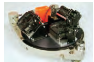
Figure 3. The DLR-3k three-camera system makes use of a fan of three Canon EOS small-format digital cameras with one firing vertically and two obliquely to provide wide cross-track coverage.
