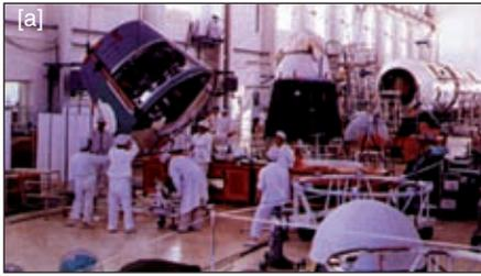
**Fig. 8 (a)** - An FSW-2 reconnaissance satellite under construction in a Chinese facility.
