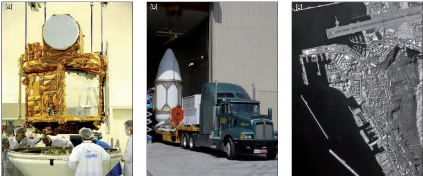
**Fig. 2 (a)** - ROCSAT-2 (now re-named Formosat-2) being lowered on to its base prior to tests being carried out on it by engineers from Taiwan's National Space Program Organisation (NSPO). The optical telescope of its pushbroom scanner is mounted on top of the main body of the satellite. (Source: NSPO)
