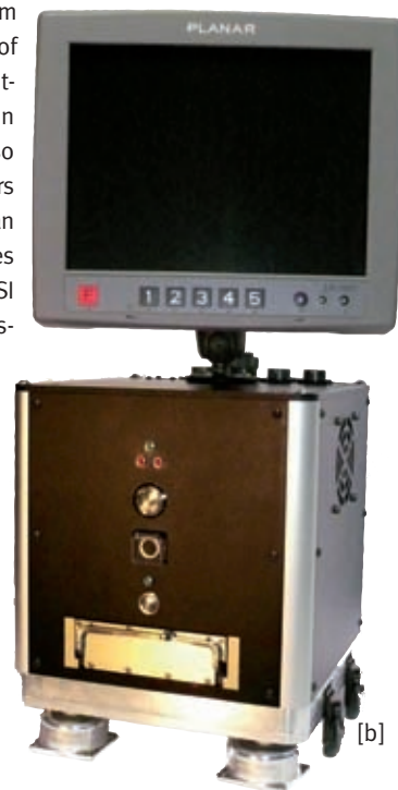
Fig. 5 – Components of the DiMAC 'Ultra-Light' medium-format airborne digital camera system, showing (a) the camera housing; and (b) the electronics case and display screen. (Source: DiMAC Systems)
