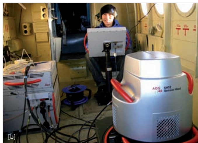
Fig. 9 – (a) This Antonov An-2 biplane is being used as a photographic aircraft by the Astanatopografiya mapping company from Kazakhstan. (b) The interior of the An-2 aircraft with a Leica Geosystems ADS40 large-format three-line pushbroom stereo-scanner in the foreground. (Source: Astanatopografiya)
