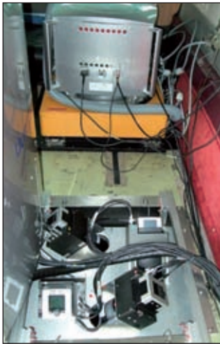
Fig. 6 – This multiple camera system comprises four IGI DigiCAM medium-format digital cameras. Each camera is acquiring oblique aerial photos at angles of 45 degrees to the vertical. Two of the cameras point in opposite directions cross-track, while the other two point in opposite directions along the flight line. In the background is a Vexcel UltraCam large-format digital camera that acquires vertical aerial photography simultaneously. (Source: Geokosmos)
