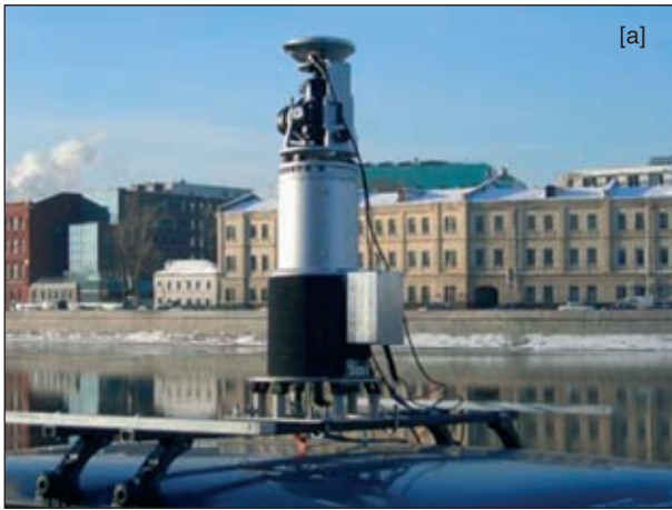
Fig. 6 - A mobile laser scanning system based on a Riegl ground-based laser together with a supplementary GPS in use for city modelling in Moscow. (Source: Riegl)
