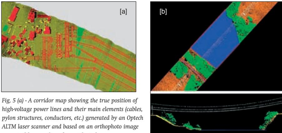
Fig. 5 (a) - A corridor map showing the true position of high-voltage power lines and their main elements (cables, pylon structures, conductors, etc.) generated by an Optech ALTM laser scanner and based on an orthophoto image generated by a medium-format digital camera.
