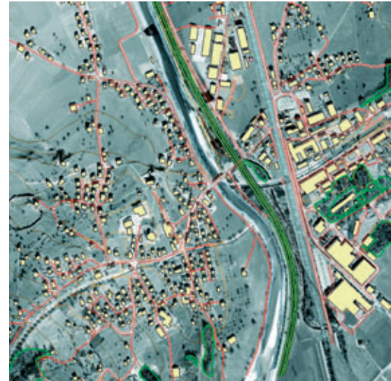
The Feature Analyst extension has been produced in collaboration with Visual Learning Systems (VLS). This aerial image of the Altdorf area in Switzerland shows the vectors defining roads, buildings, etc. that have been extracted using Feature Analyst.
