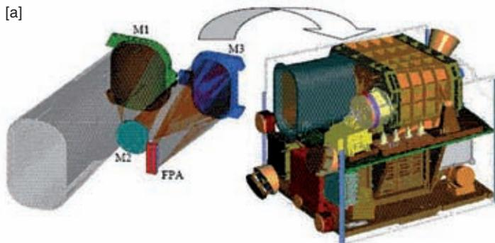
**Fig. 3 (a)** - The three-mirror anastigmatic (TMA) telescope showing the mirrors (M1, M2 & M3) and the focal plane array (FPA) and their relationship to the overall construction of the JSS-56 spaceborne scanner on which it is mounted.
