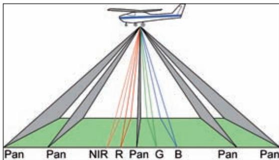
**Fig. 7** - The geometry of the nine-line arrangement of the linear arrays used in the HRSC-AX and JAS 150 pushbroom line scanners showing their angular positions and ground coverage. [Pan = Panchromatic; B = Blue; G = Green; R = Red; NIR = Near Infra-red] (Drawn by M. Shand)
