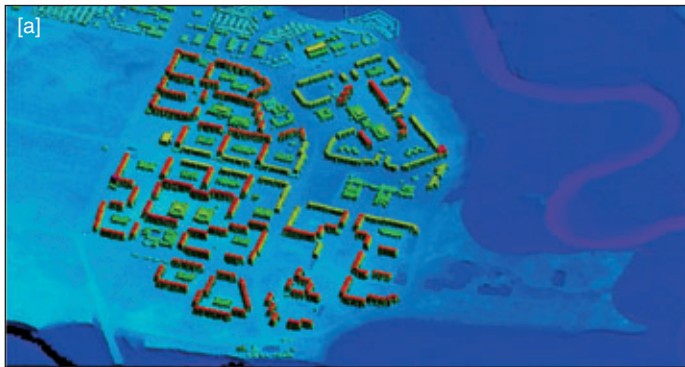
(a) Digital Surface Model (DSM) of part of the town of Novyi Urengoi located in the Tyumen region of Western Siberia. This DSM has been derived from airborne laser scanning carried out by the Geokosmos company for the Gazprom organization during its mapping of the large area of gas fields located in this region.
