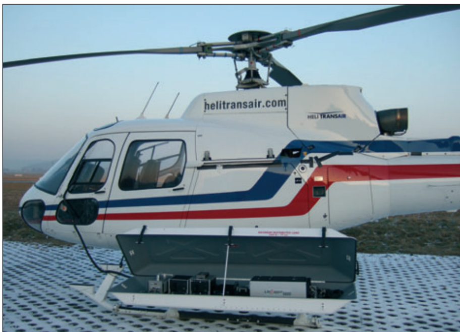
A helicopter is being used by the Hansa Luftbild mapping company to acquire terrain elevation data utilizing an IGI LiteMapper 5600 airborne laser scanning system mounted externally in a Helipod box. (Source: IGI)
