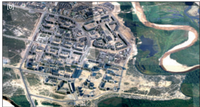
(b) The corresponding image of the same area formed by merging the elevation data of the DSM with the image data collected (in colour) simultaneously by a Rollei medium-format airborne digital camera. (Source: Geokosmos)
