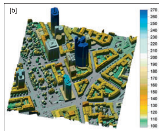
(b) A 3D perspective view of part of the centre of the city of Frankfurt that has been constructed from airborne lidar elevation data acquired by an ALS50 laser scanner. (Source: Astec)
