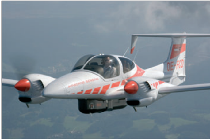
(a) This twin-engine Diamond DA42 MPP (Multi Purpose Platform) aircraft has been equipped with a specially built pod fitted below the aircraft to accommodate the Riegl LMS-S560 airborne scanning system.
