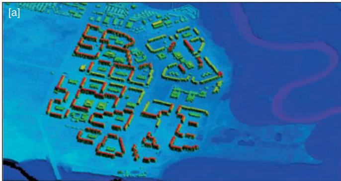
(a) Digital Surface Model (DSM) of part of the town of Novyi Urengoi located in the Tyumen region of Western Siberia. This DSM has been derived from airborne laser scanning carried out by the Geokosmos company for the Gazprom organization during its mapping of the large area of gas fields located in this region.
