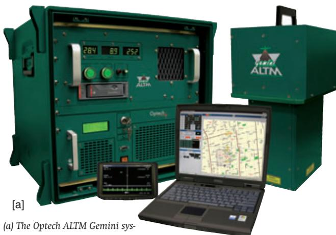
[a] The Optech ALTM Gemini system that was introduced at INTERGEO 2006. At back left is the case containing the control electronics; at back right is the scanning laser unit; at the front are the monitoring and operator control screens. (Source: Optech)
