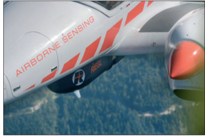
(b) A close-up view of the belly pod containing the Riegl laser scanning system attached to the DA42 MPP aircraft. (Source: Diamond Airborne Sensing)
