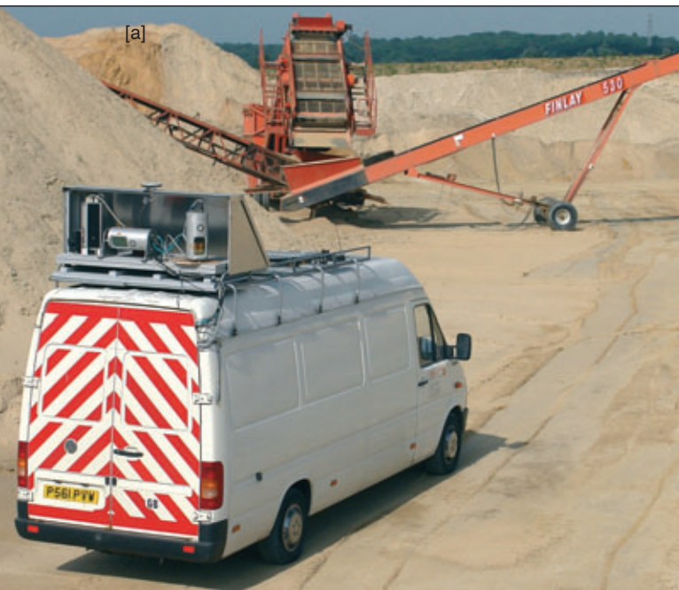
Fig. 6 - (a) A StreetMapper van equipped with laser scanners mounted on the vehicle's roof rack. (b) Components of a StreetMapper system mounted on the roof rack of a vehicle showing the laser scanners, TERRAcontrol DGPS/IMU unit and the GPS antenna. (c) The displays associated with the StreetMapper system mounted on the front fascia (dash-board) of the van.
