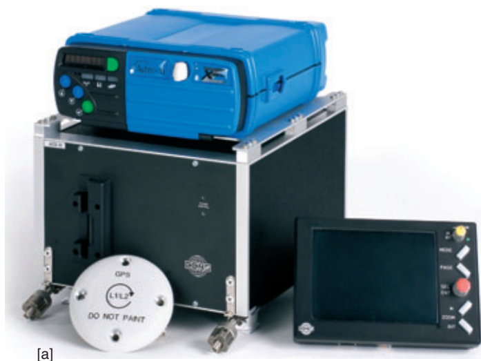
Fig. 1 - (a) A CCNS4 airborne navigation and guidance system showing the main Computer Control Unit (CCU) with the blue Ashtech GPS unit sitting on top of it and the round white GPS antenna placed in front of it. The Command & Display Unit (CDU) with its TFT screen is situated to the right. (b) - The pilot of this survey aircraft is flying it on its planned track using the CCNS4's Command & Display Unit (CDU) fitted above the aircraft's main instrument panel.
