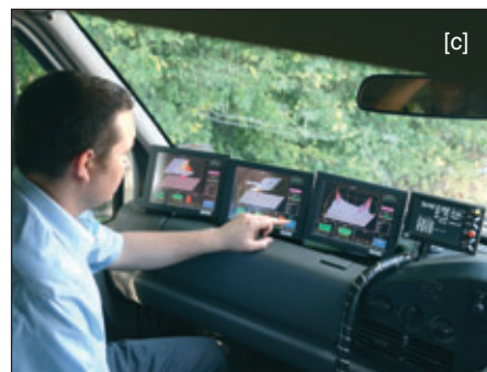
Fig. 6 - (a) A StreetMapper van equipped with laser scanners mounted on the vehicle's roof rack. (b) Components of a StreetMapper system mounted on the roof rack of a vehicle showing the laser scanners, TERRAcontrol DGPS/IMU unit and the GPS antenna. (c) The displays associated with the StreetMapper system mounted on the front fascia (dash-board) of the van.
