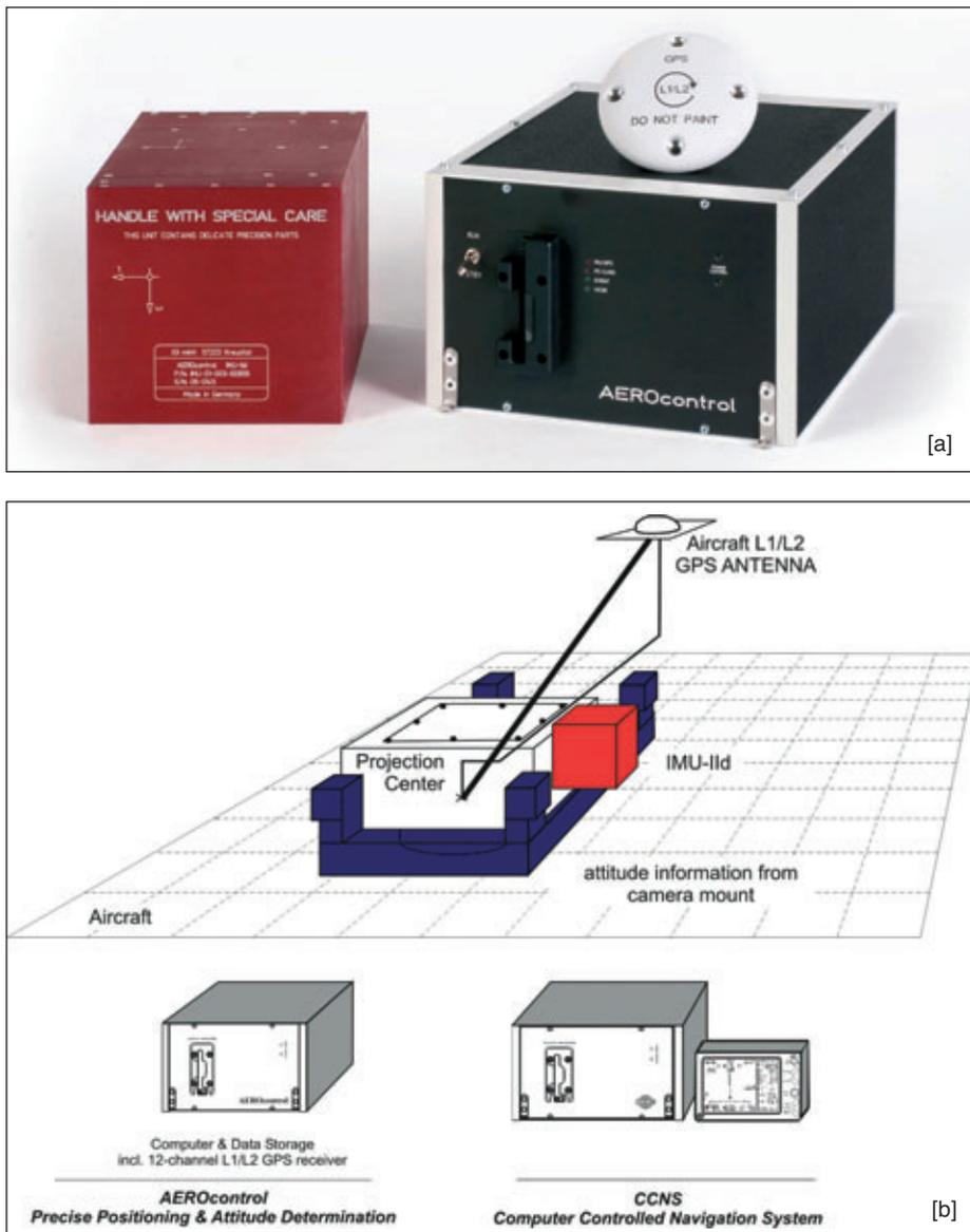
Fig. 2 - (a) An AEROcontrol-Iid system with the integrated DGPS/IMU unit housed in the red box on the left while the computer and data storage unit is on the right with the white round GPS antenna sitting on top of it. (b) - The diagram shows the AEROcontrol lever arm correction that relates the position of the GPS antenna to the projection centre of the aerial camera.
