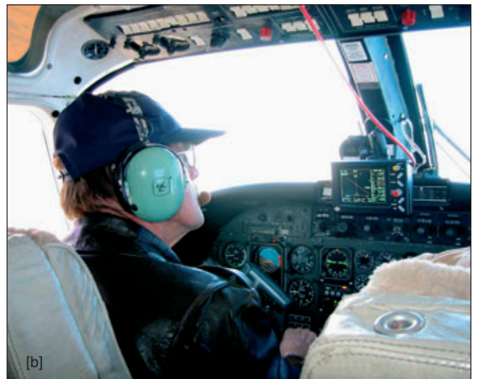
Fig. 1 - (a) A CCNS4 airborne navigation and guidance system showing the main Computer Control Unit (CCU) with the blue Ashtech GPS unit sitting on top of it and the round white GPS antenna placed in front of it. The Command & Display Unit (CDU) with its TFT screen is situated to the right. (b) - The pilot of this survey aircraft is flying it on its planned track using the CCNS4's Command & Display Unit (CDU) fitted above the aircraft's main instrument panel.
