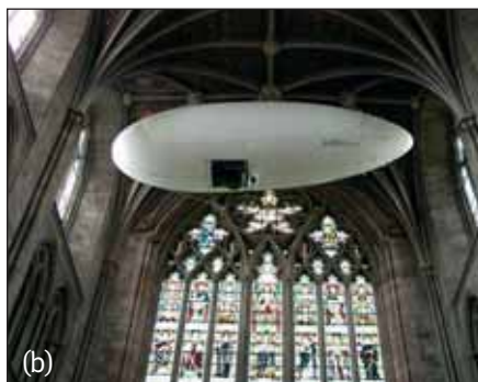
Figure 4 (a) - A powered balloon operated by Skycell Ltd. acquiring photography in Wells Cathedral in Somerset, England. The ducted propellers can be seen on each side of the balloon with the digital camera on its mount hanging down from the centre of the main envelope of the balloon. (Source: Dr. Szymanski, University of York)
