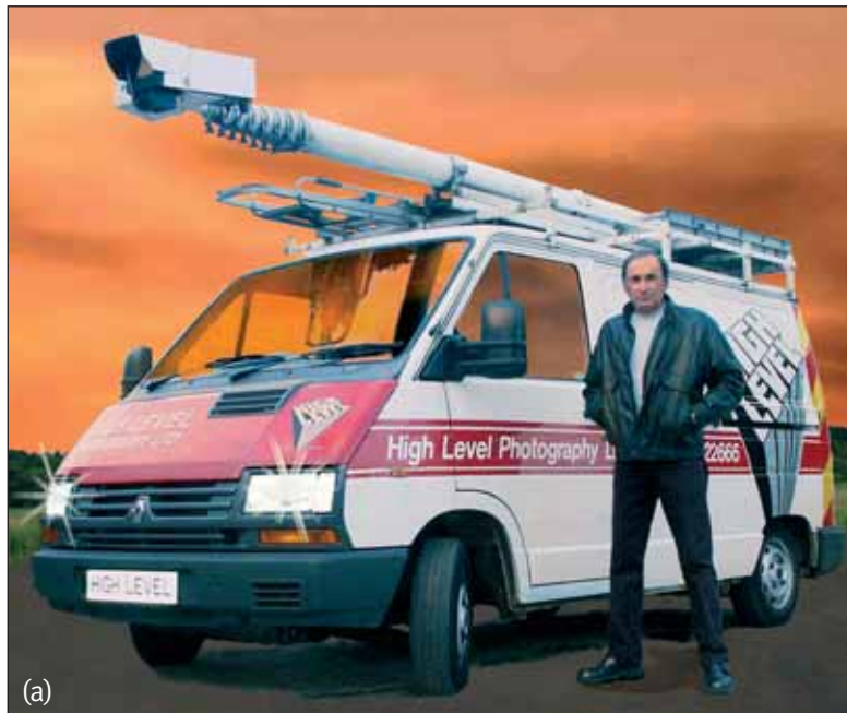
Figure 1 (a) - A mobile van equipped with a 80 ft. (24m) telescopic mast that is used to obtain elevated (aerial) photography using a film, digital or video camera. This particular van belongs to High Level Photography Ltd. based in Guildford, Surrey. The company owner, Keith Hallam is standing in front of the vehicle. (Source: High Level Photography)
