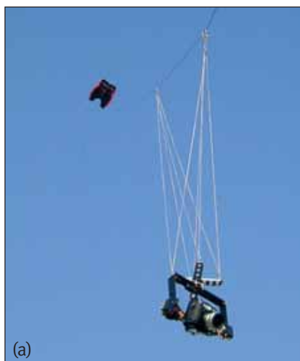
Figure 5 (a) - Aerial photography is being acquired in this photo using a Flowform kite being flown by Scott Haefner of Palo Alto, California. The Nikon digital camera is attached to the main tether line using a set of Picavet suspension cables that carries the cross-shaped base plate and the camera mount. (Source: Scott Haefner)
