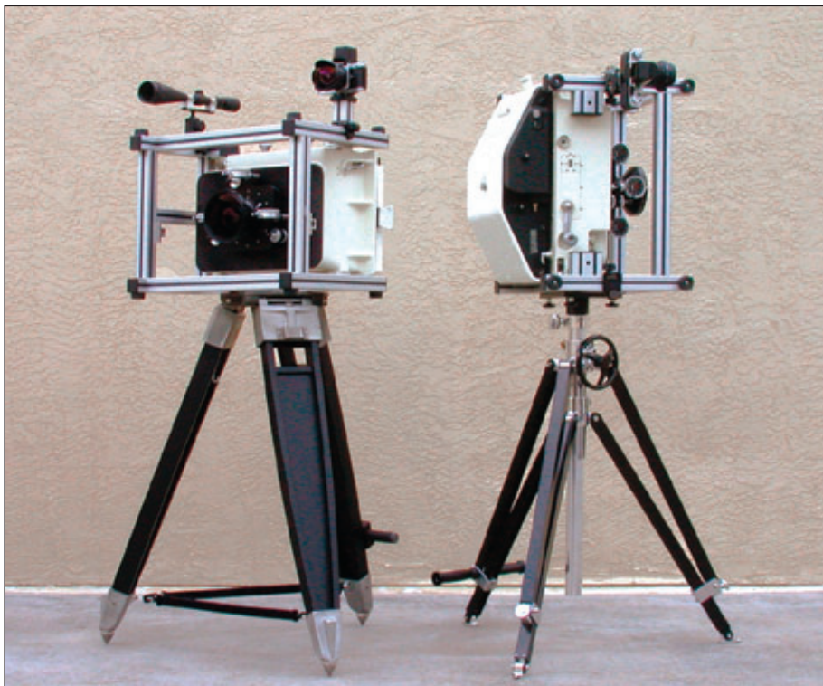
Figure 1b: Two different versions of the Fairchild large-format film cameras that have been modified for use in the Gigapxl Project - with the long (18 inch) side set in the horizontal position in the example on the left of the picture and set in the vertical position in the example on the right. (Source: Gigapxl Project)
