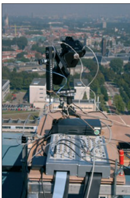
Figure 2c: The Nikon D1x small-format digital camera with its motorized pan-and-tilt head and motion controller hardware mounted on the parapet of the 100m high Electrical Engineering building of the Delft University of Technology to order to acquire the photos of the town. (Source & Copyright: TNO)
