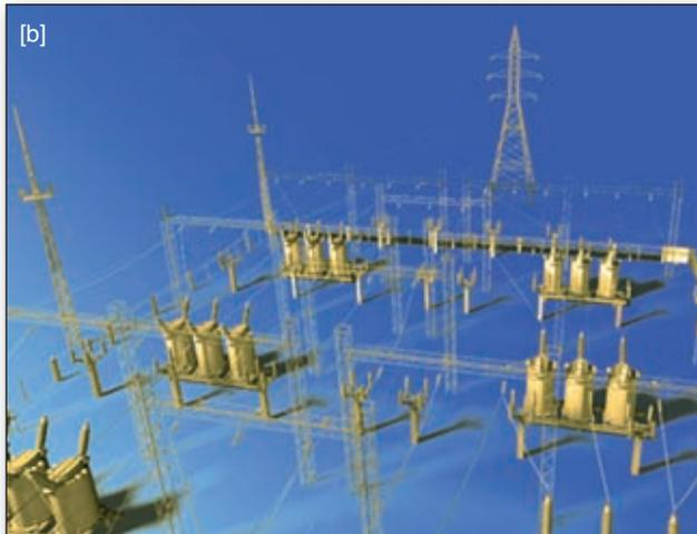
**(b)** - A perspective 3D model of an electric power sub-station based on terrestrial laser scan data.
