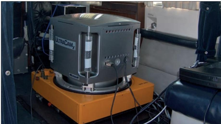
Figure 4 – This example of a Vexcel UltraCam-X large-format digital frame camera, mounted on a Somag GSM3000 gyro-controlled platform, is operated by the Croatian company, Geofoto, based in Zagreb. [Source: Geofoto]
