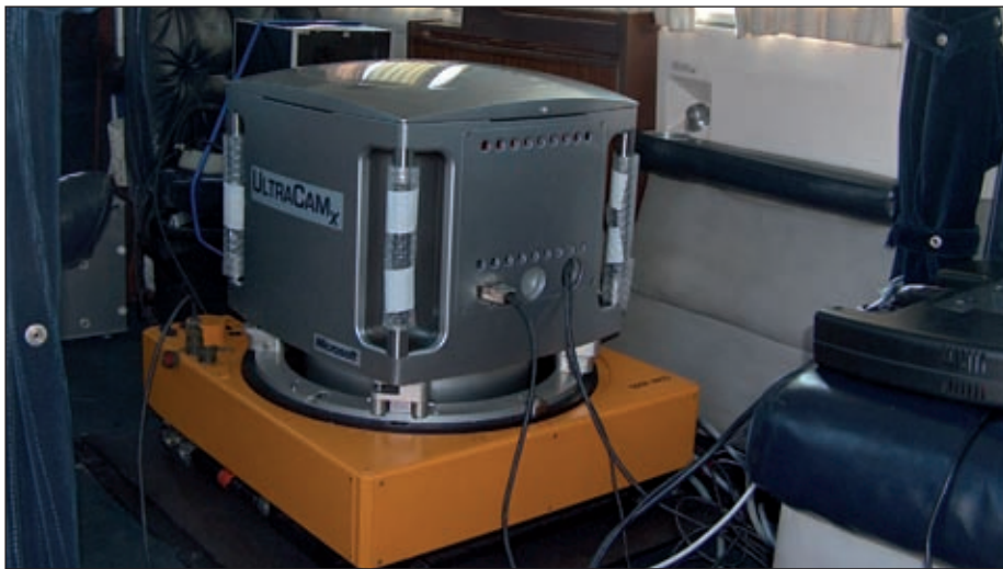
Figure 4 – This example of a Vexcel UltraCam-X large-format digital frame camera, mounted on a Somag GSM3000 gyro-controlled platform, is operated by the Croatian company, Geofoto, based in Zagreb. [Source: Geofoto]
