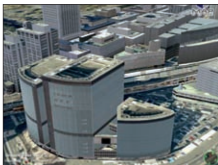
Figure 3 – A 3D perspective view of part of the city of New Delhi based on a digital model formed from stereo-photogrammetric measurements of the buildings with the textures added from a photographic library.
