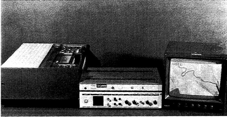
Fig. 11 - Video-based monocomparator
