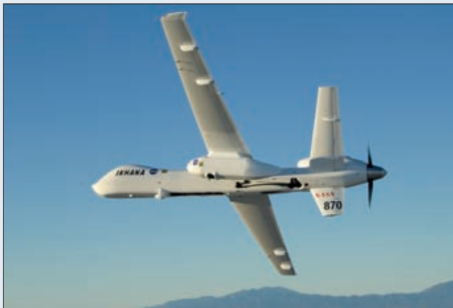
Fig. 2A The NASA Ikhana UAV, which is a modified Predator-B unmanned aircraft, is shown in flight.
