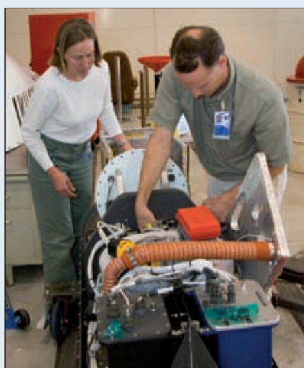
Fig. 2C The Autonomous Modular Scanner (AMS) thermal-IR imager is being loaded into the under-wing pod prior to being mounted on the wing of the Ikhana UAV.
