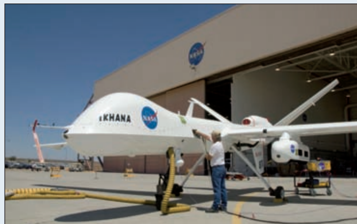
Fig. 2B The NASA Ikhana UAV is being checked out on the ground – note the under-wing pod which houses the imager.
