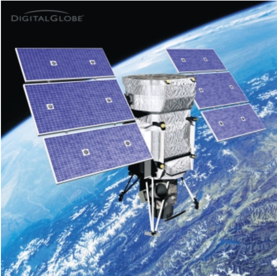
Figure 8. An artist's impression of the new WorldView high-resolution satellite being constructed for DigitalGlobe. It is designed to produce imagery with 0.5m (pan) and 2.0m (multi-spectral) ground pixel [GSD] sizes respectively. (Source: DigitalGlobe)
