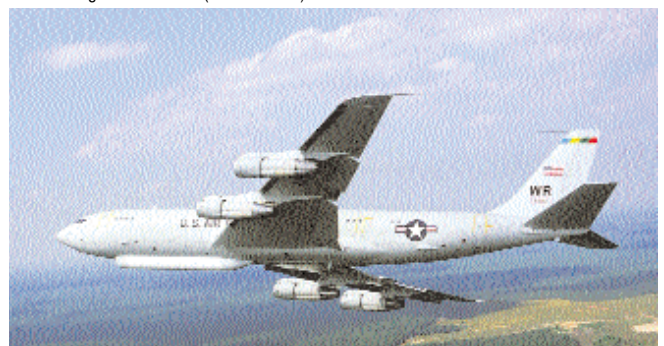
Figure 2: (b) The USAF's E-8 J-STARS aircraft based on a re-manufactured Boeing 707-300 airframe. The 12-metre (40-foot) canoe-shaped radome hung under the aircraft's forward fuselage houses a 7.3-metre (24-foot) long side-looking radar antenna. (Source: USAF)
