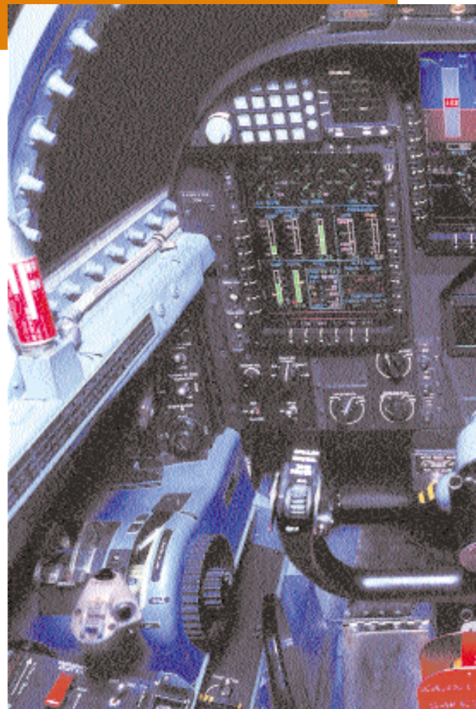
Figure 1(b): The new 'all-glass' cockpit of the U-2S aircraft equipped with large multi-function displays and modern avionics. (Source: Lockheed Martin)
