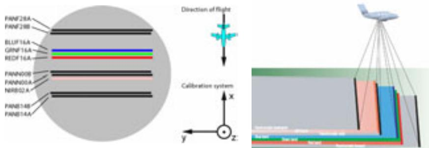
Again **offsets** are created – different lines are being imaged on the ground at the same instant of time
