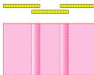
Top (yellow part) – shows three linear arrays mounted in the focal plane of a digital line scanner;
