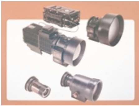
(a) Barr & Stroud IR-18 frame scanner with five alternative lenses giving different magnifications and fields of view. (b) Agema ThermoVision 1000 frame scanner equipped with an internal lens turret allowing either narrow (5°) or wide angle (20°) fields of view.
