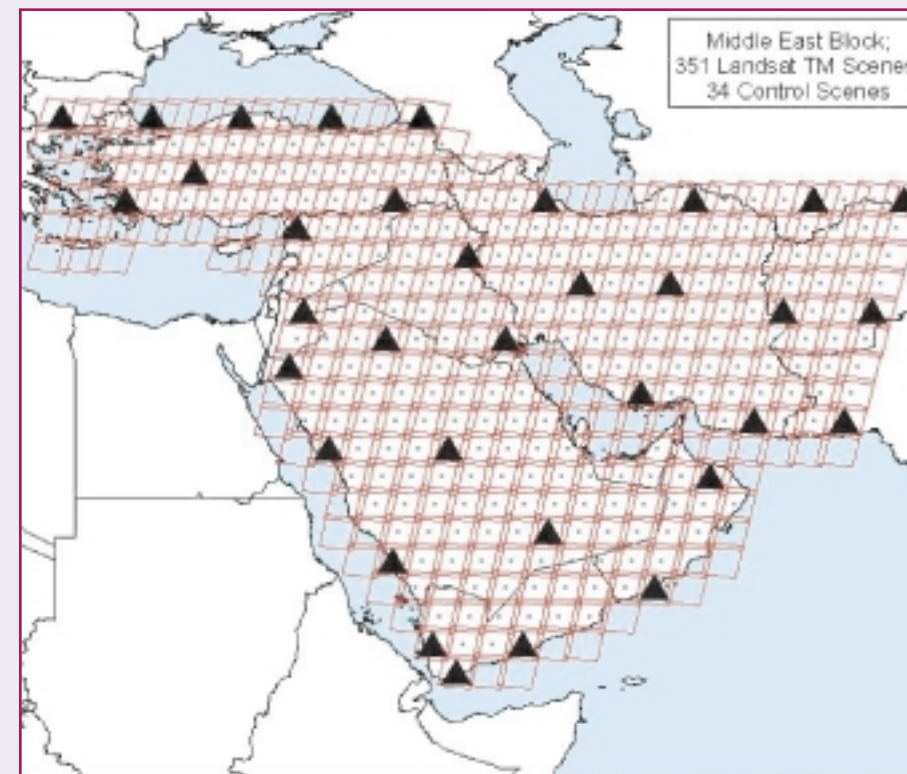
The Middle East block of EarthSat's GeoCover-Ortho Project comprising 351 Landsat TM scenes fitted to 34 control scenes containing ground control points (GCPs). These were triangulated and adjusted simultaneously as a single block to provide control points for the subsequent ortho-rectification operation. (Courtesy EarthSat)
