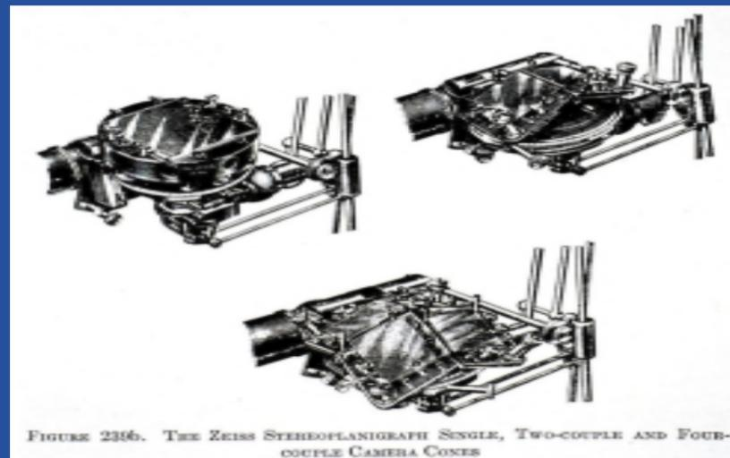
The single, two-coupled and four-coupled plotting cones used with the Stereoplanigraph. (Source: Talley - "Engineering Applications of Aerial & Terrestrial Photogrammetry", 1938)
