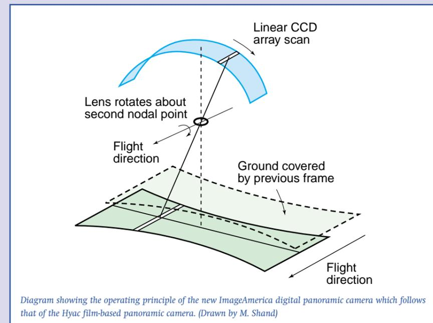
Diagram showing the operating principle of the new ImageAmerica digital panoramic camera which follows that of the Hyac film-based panoramic camera. (Drawn by M. Shand)
