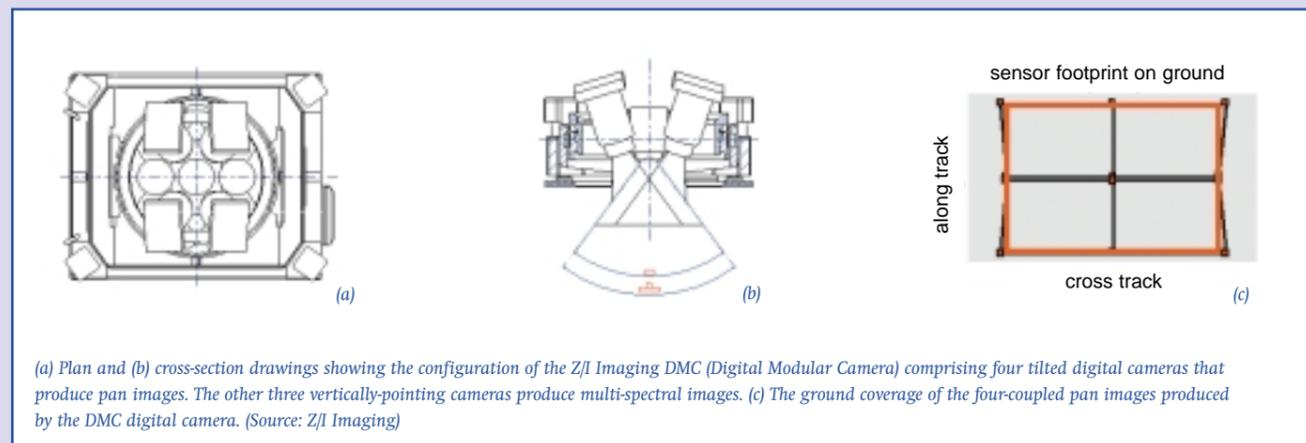
(a) Plan and (b) cross-section drawings showing the configuration of the Z/I Imaging DMC (Digital Modular Camera) comprising four tilted digital cameras that produce pan images. The other three vertically-pointing cameras produce multi-spectral images. (c) The ground coverage of the four-coupled pan images produced by the DMC digital camera. (Source: Z/I Imaging)
