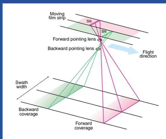
Diagram showing the concept of the shutterless airborne film strip camera providing stereo-coverage of the ground. (Drawn by M. Shand)
