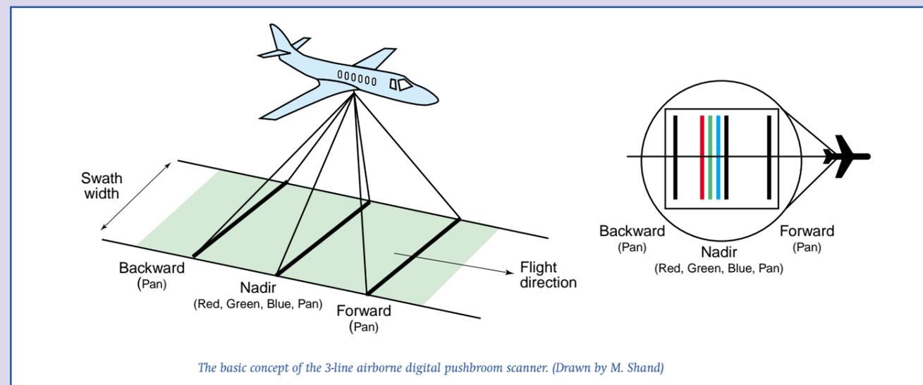
The basic concept of the 3-line airborne digital pushbroom scanner. (Drawn by M. Shand)
