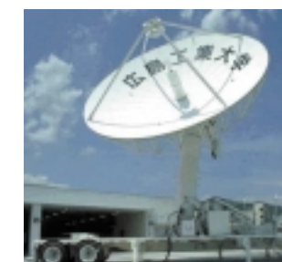
The 7.3m diameter antenna system from Datron/Transco mounted on a 40 ft. (9m) long trailer that forms part of the transportable ground receiving station supplied by the Vexcel Corporation to the Hiroshima Institute of Technology in Japan. (Source - Vexcel Corporation)
