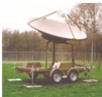
The trailer-mounted antenna of the RAPIDS transportable station with its 2.6m diameter dish antenna. The system uses two hydraulically driven rams to provide a smooth precision-controlled tilt movement of the dish during the automatic tracking of satellites such as SPOT and ERS. The trailer can be set up on jacks while operating from a fixed position. (Source - NRI)
