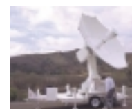
The 3.6m diameter tracking antenna mounted on its trailer that forms part of the Eagle Vision transportable ground receiving station operated by U.S. military forces. (Source - Datron/Transco)
