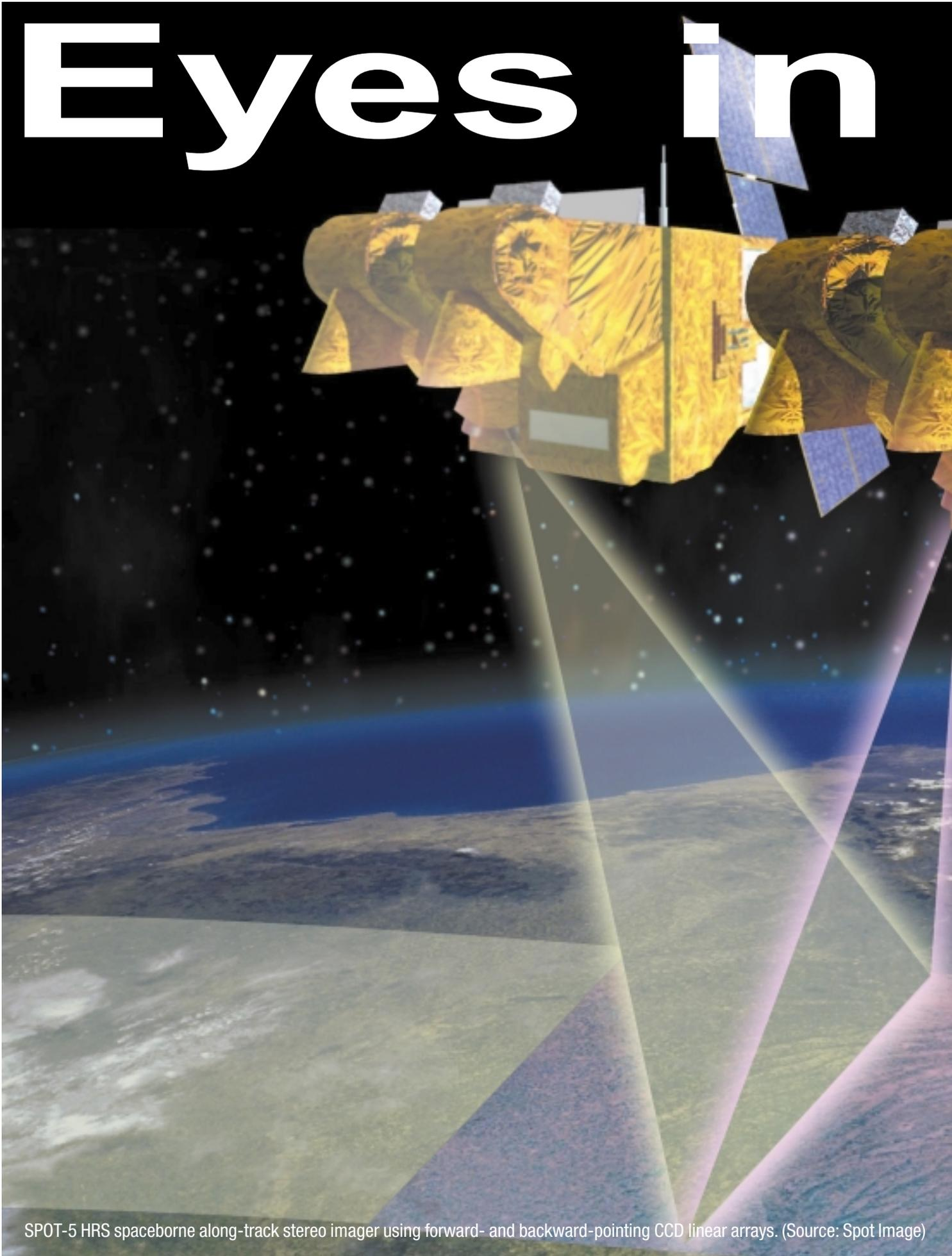
SPOT-5 HRS spaceborne along-track stereo imager using forward- and backward-pointing CCD linear arrays. (Source: Spot Image)
