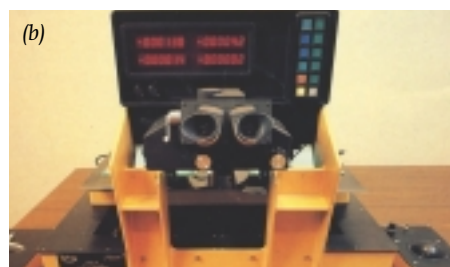
Figure 1: (a) The APPS-I analytical photogrammetric instrument from the 1970s. The photogrammetric solution was provided on a point-by-point basis using software running on a Hewlett-Packard desktop calculator. (b) The APPS-IV analytical plotter from the 1980s.
