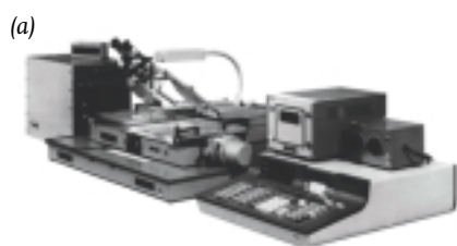
Figure 1: (a) The APPS-I analytical photogrammetric instrument from the 1970s. The photogrammetric solution was provided on a point-by-point basis using software running on a Hewlett-Packard desktop calculator. (b) The APPS-IV analytical plotter from the 1980s.
