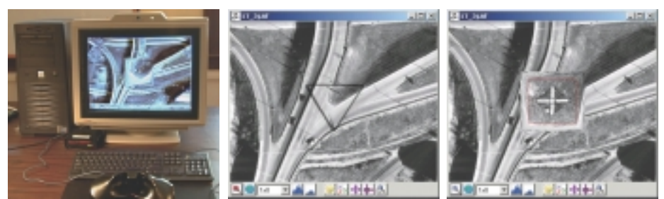
Figure 3: (a) The new Kork Digital Stereo Plotter (KDSP) designed for digital vector map production with the Idelix lensing tool located in the centre of the display. (b) The KDSP display screen before the Idelix "lens" has been switched on. (c) The KDSP display screen with the Idelix "zoom lens" switched on.
