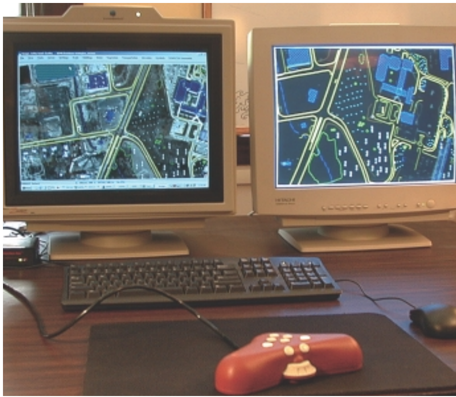
Figure 2: A SoftPlotter digital photogrammetric workstation (DPW) running in a twin-screen configuration with the SoftMouse used for 3D measurement in the stereo-model in the foreground.
