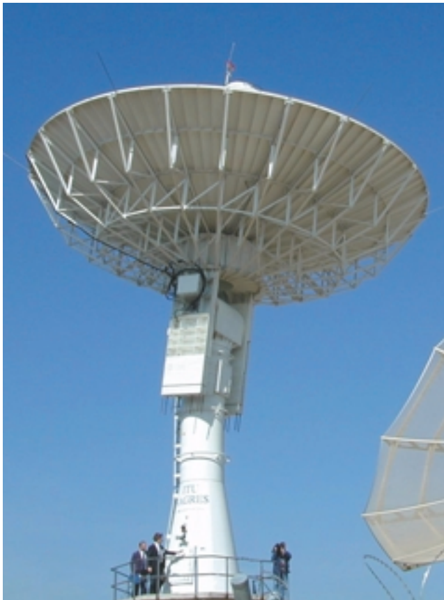
Fig. 2: The 13m diameter antenna of the newly constructed ground receiving station installed at Istanbul Technical University (ITU). (Source: Datron Advanced Technologies)
