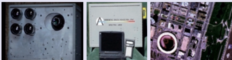
Fig.3: (a) The Spectra-View airborne digital multi-spectral camera manufactured by Airborne Data Systems Inc. This example is equipped with five lenses and CCD areal arrays - with four of these optical units covering the blue, green, red and near infra-red bands, while the fifth covers the thermal infra-red band. (b) The Spectra-View camera seen from the back, complete with the laptop computer and hand controller used on-board the aircraft during flight. (c) A multi-spectral frame image covering part of Downtown St.Louis that was acquired during the ASPRS Conference. The image includes the Busch baseball stadium and the Gateway Arch. (Source: Airborne Data Systems Inc.)
