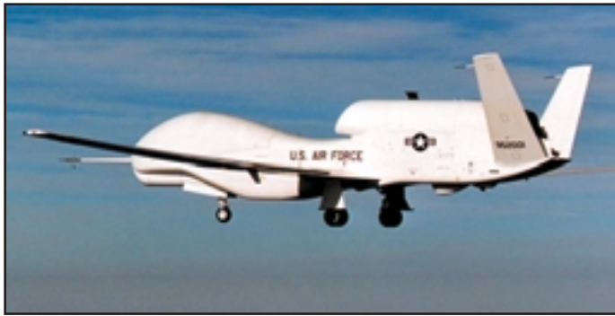
(A): Northrop Grumman Global Hawk high-altitude, long-endurance (HALE) UAV. (Source: Northrop Grumman)
