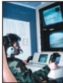
(C): Pilot flying the UAV from the ground station. (Source: General Atomics)
