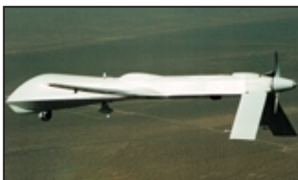
Left: General Atomics Predator propeller-driven UAV with the imager turret fitted below the nose of the aircraft. Right: The gyro-stabilised turret containing the EO/IR imagers fitted to the underside of the nose of the General Atomics Predator UAV. (Source: General Atomics)
