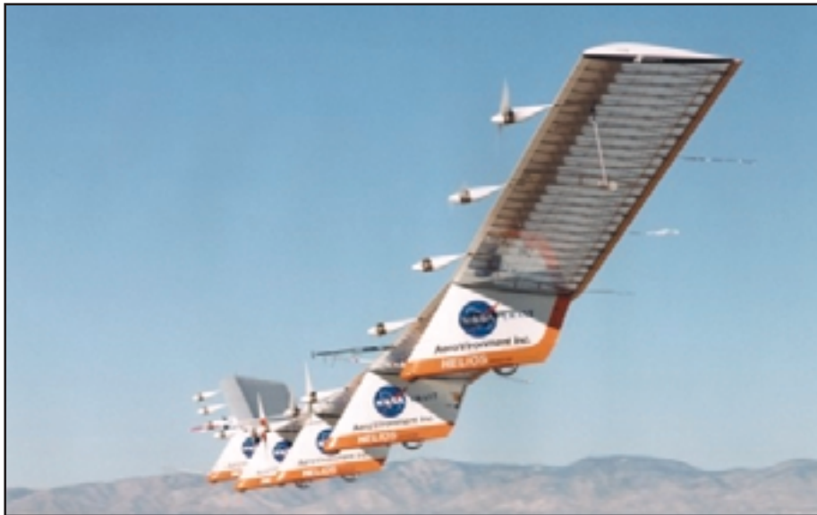
The prototype of the Helios solar-powered high-altitude flying wing UAV lands on the lake bed near Dryden Flight Research Center at Edwards Air Force Base in California. (Source: NASA)
