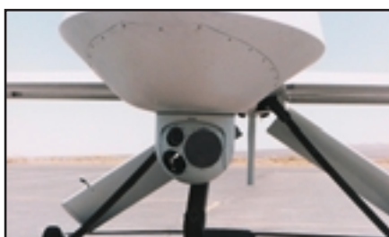
Left: General Atomics Predator propeller-driven UAV with the imager turret fitted below the nose of the aircraft. Right: The gyro-stabilised turret containing the EO/IR imagers fitted to the underside of the nose of the General Atomics Predator UAV. (Source: General Atomics)
