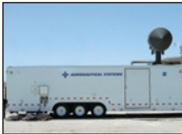
(B): NASA's mobile ground control and receiving station with the parabolic tracking antenna on top of the van providing the line-of-sight radio link to the UAV. (Source: General Atomics)
