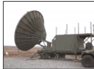
(D): The Trojan Spirit II ground station receiving the image data from the UAV via a communications satellite. (Source: U.S. Army)
