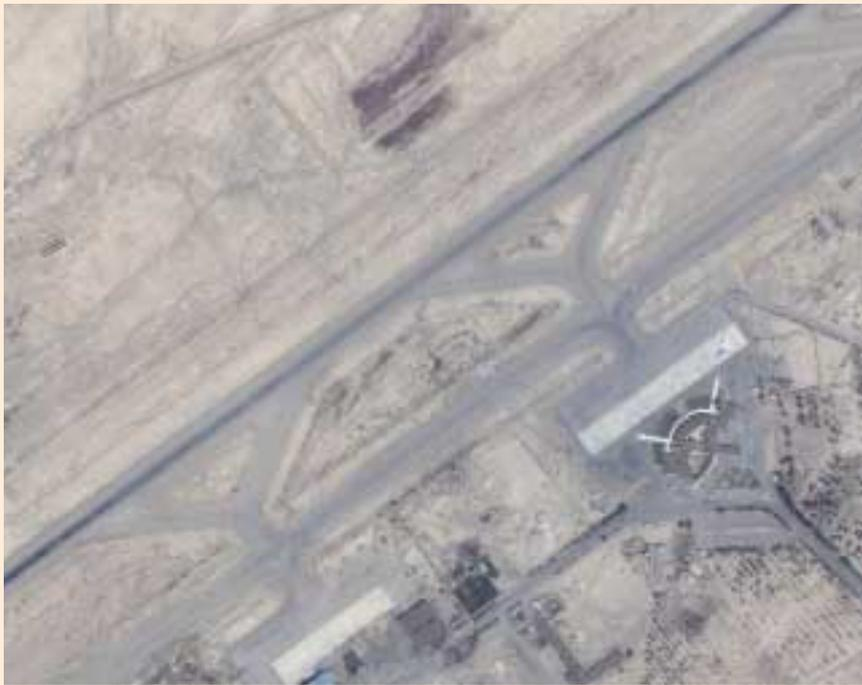
Figure 2: Images of Kandahar Airport (a) before, and (b) after the air attacks by US aircraft. The damage to the airport's runway, taxiways and revetments can be clearly seen. The images were acquired by the IKONOS satellite on 23 April and 10 October 2001 respectively. (Source and copyright: Space Imaging)
