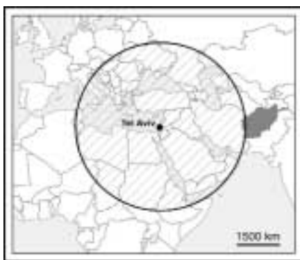
Figure 3: Diagram of the ground coverage of the Israeli ground station near Tel Aviv for the direct reception of EROS-A1 imagery. (Drawn by Mike Shand)
