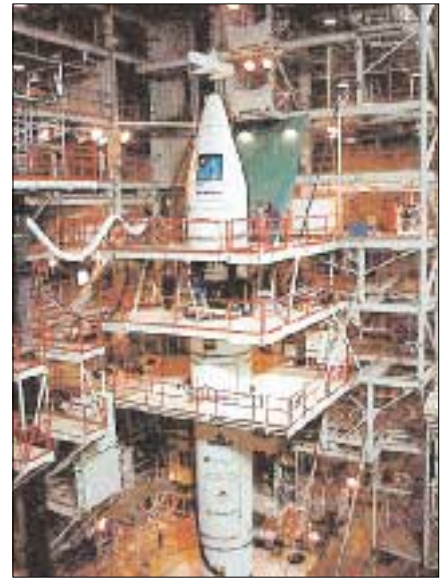
Figure 2: The IKONOS satellite being fitted to its Athena rocket prior to launch. (Source: Space Imaging)
