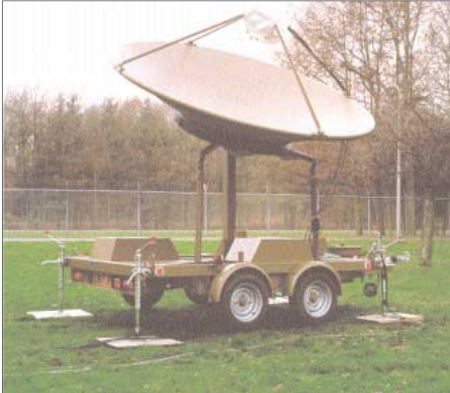
Figure 5: The trailer-mounted antenna of the RAPIDS transportable ground receiving station with its 2.6 metre diameter dish antenna. (Source: NRI)
