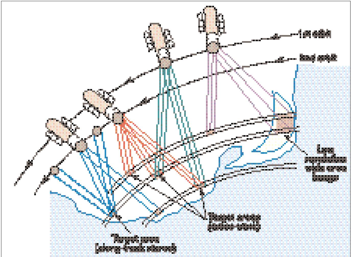
Figure 3(b): The different operational modes of the KH-12 satellites. (Drawn by M. Shand; adapted from diagrams by C.A. Vick of the Federation of American Scientists)
