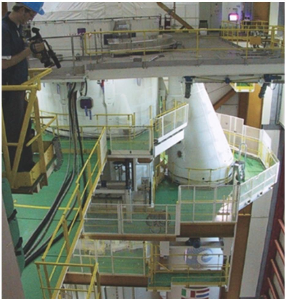
Figure 3: The Ariane-5 launcher awaiting the arrival and fitting of Envisat. (Source: Astrium)
