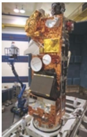
Figure 1: (a) A diagram showing the overall construction of Envisat and the positions of the antennae of the various imagers and other instruments that are mounted on the satellite. (b) The corresponding photograph of Envisat taken while under test at ESA-ESTEC. (Source: ESA-ESTEC)
