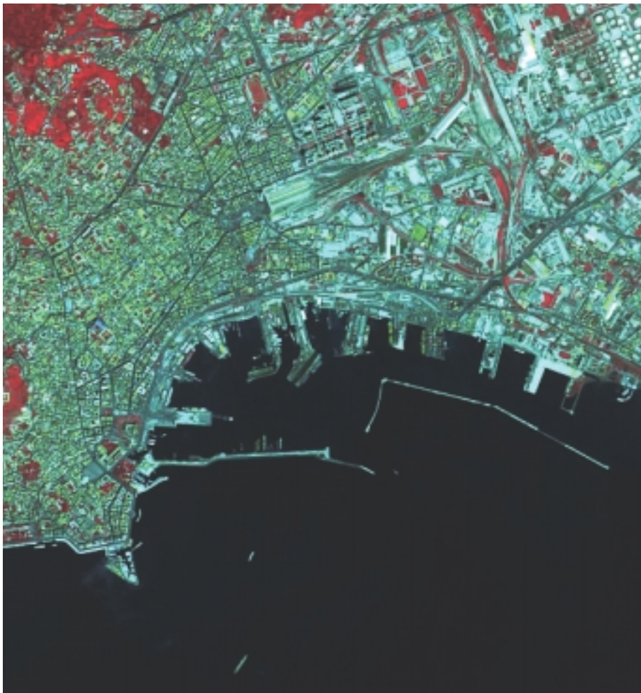
Figure 2: A multi-spectral, false-colour image of the city and port of Naples, Italy. The image was acquired with a 10m ground pixel size by the newly launched SPOT-5 satellite. (Source: SPOT Image).
